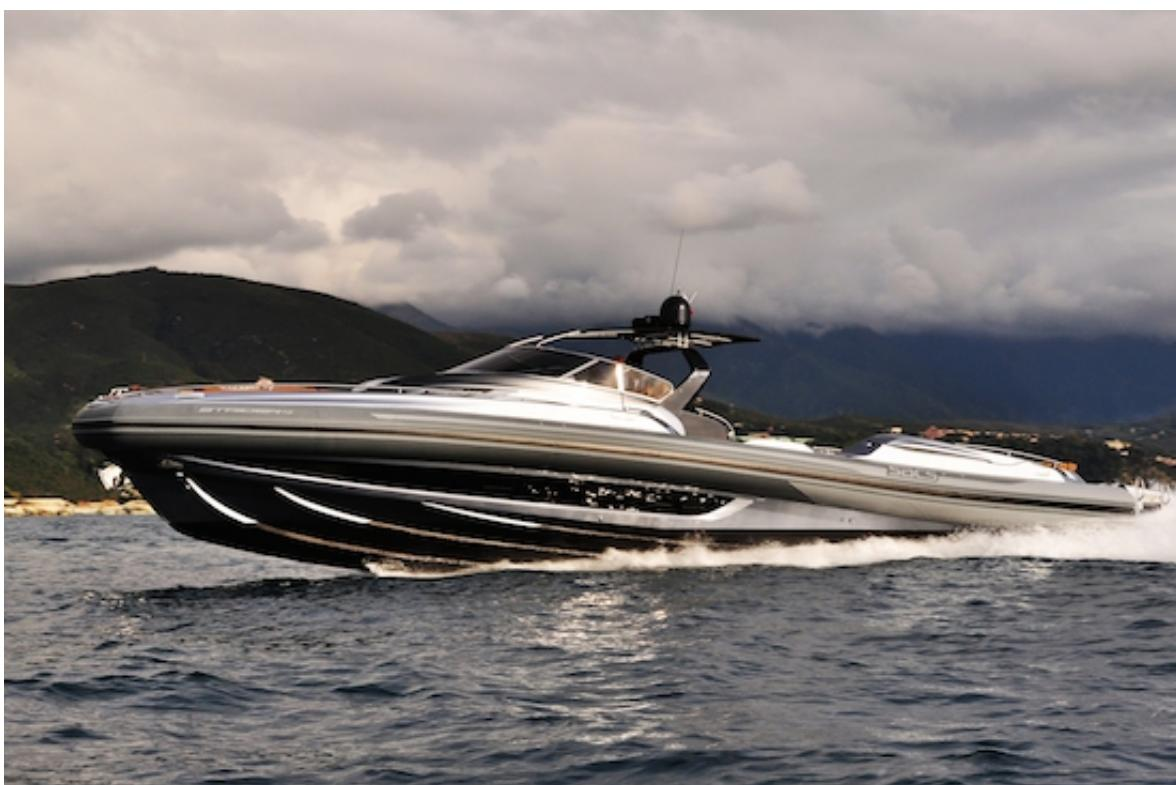
The Strider 19 features a deep-V hull, low center of gravity, and her large tubes allow for fast cruising in all sea conditions. She is powered by twin 1,150 hp Caterpillar engines, which enable the yacht to reach a top speed of 50 knots, and a cruising speed of about 45 knots.
